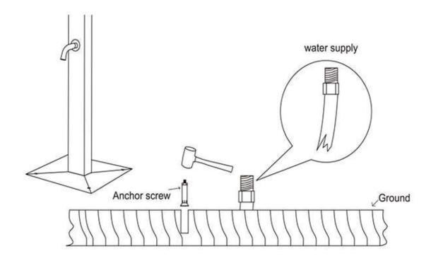
Secure the base plate using the 4 x Dyna bolts on top of the pipes, with pipes protruding through the center of the base 8. Remove the back panel of the shower
