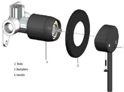
1. Fix the body of the mixer to a suitable fixing plate or noggin. Ensure the mixer is level and will have enough of the body exposed to install the plate (part 2) and handle (part 4).
