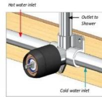
3. Remove the protective covers and carefully slide the back-plate (part 2) over the mixer/diverter bodies until it is firm against the wall (It is recommended to apply a clear sealant behind the back plate to ensure water cannot run behind the plate).
